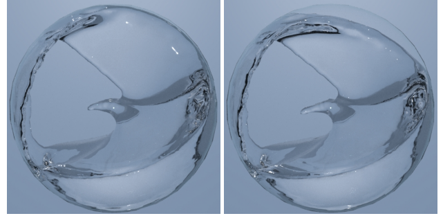
Figure 3.2: A selected frame from two simulations of a 3D scenario of liquid splashing inside a spherical boundary. Left: Without separating solid wall boundary conditions, the liquid adheres to the top of the sphere. Right: With separating solid wall boundary conditions, the liquid separates naturally.
