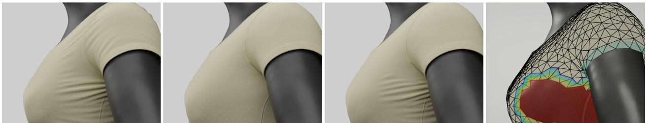
Figure 1: Mixing yarns and triangles to efficiently predict fitting details of a shirt. From left to right: simulation result with a full-yarn model, a triangle-only model, and our method, and mixed discretization with triangles and yarns. The triangle-based model misses all the detailed wrinkling of the yarn-based model. We select a region of interest on this triangle-based model, we enrich it with yarns, and the mixed result reproduces the wrinkles of the full model. Wrinkles outside the region of interest are not captured, as expected.
