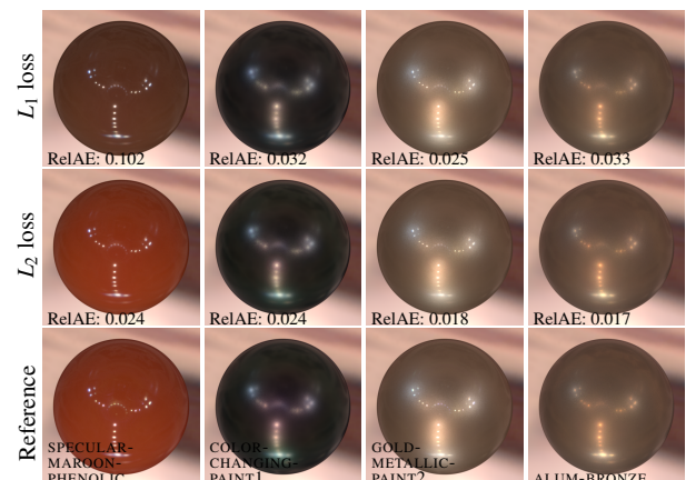
Figure 4: Comparison between L_1 loss and L_2 loss in designing the loss function. The corresponding Relative Absolute Error (RelAE) for each reconstructed result is reported.
