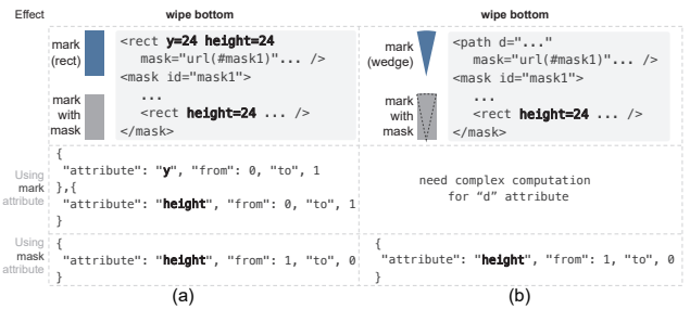
Figure 3: Implementation the animation effects by using mask attributes (a,b), highlighted in bold. (a) using one mask attribute allows us to achieve the “wipe bottom” effect instead of using the two attributes; and (b) for the marks defined by SVG path element, using the mask attribute allows us to achieve the animation effect easier than by using mark attributes.
