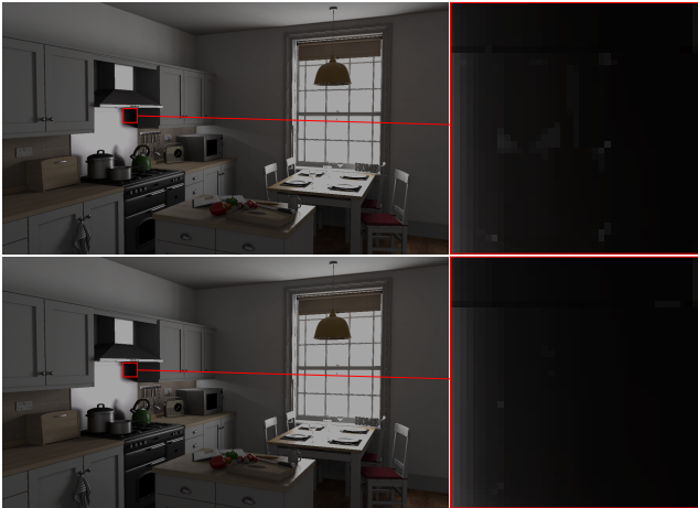
Figure 9: Light leaks can be caused by insufficient sampling in high rank areas (top). Increasing the number of verification samples improves this (bottom).
