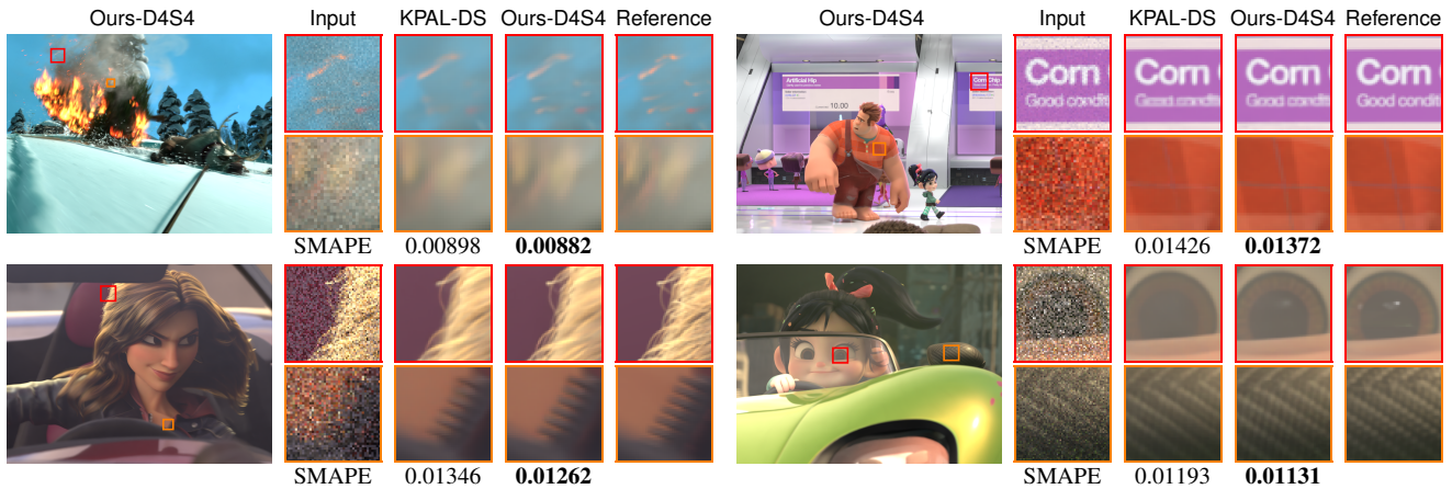
Figure 7: Comparison with KPAL on HYPERION test set. Our method can improve the reconstruction quality of details. © 2021 Disney
