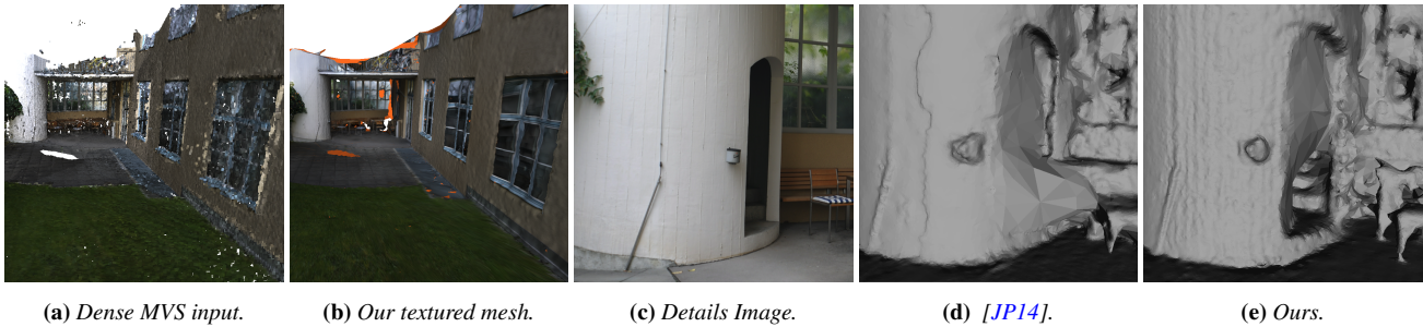
Figure 7: Qualitative Results on ETH3D. Our mesh reconstruction method takes as input a dense MVS point cloud (a) and produces a mesh (b), simultaneously preserving fine details and completing missing parts (here textured with [WMG14]). We represent: in (c), a cropped image of a detail from the terrace scene of the ETH3D benchmark [SSG*17]; in (d), the reconstruction by Jancosek and et al. [JP14]; and in (e), our reconstruction. Notice the missing staircase and spurious vertical pattern on the concrete wall in (d). In contrast, our method (e) reconstructs part of the staircase as well as the fine-grained wall textures.
