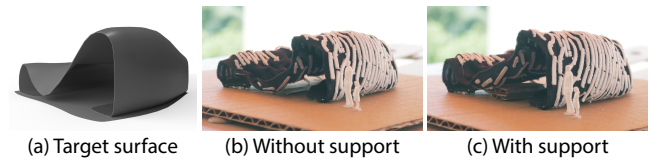
Figure 12: Limitation. Without additional support, this architectural model sags under its own weight (b). Adding a cardboard support underneath the structure brings it closer to the target surface (c).
