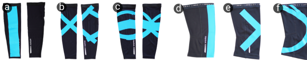
Figure 14: Fabricated Garments for user study. Line, X, and Optimal designs for elbow sleeves (a-c), and knee sleeves (d-e) respectively.
