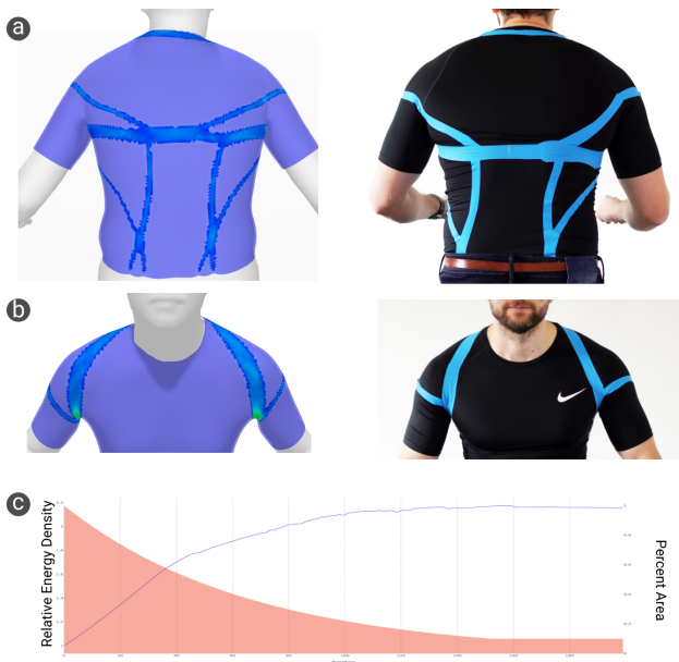
Figure 9: Optimized posture correcting shirt viewed from the back (a) and front (b). Area coverage is 10%. Note the smooth increase in energy density (c) over the optimization process.
