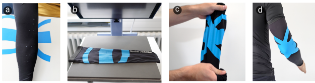
Figure 13: Garments reinforcement material (HTV) is cut (a) and transferred onto the base garment using a heat press (b). The resulting garment has high compliance (c) and can be worn as a typical sleeve (d).
