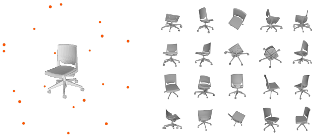
Figure 5: Left: configuration of rendering views. 20 camera positions are illustrated as red points. Right: 20 rendered images for computing FID, the image resolution is 299 \times 299 .
