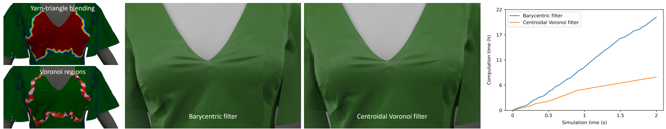
Figure 8: This figure shows an example borrowed from [CCR*20], which combines triangle-based and yarn-level cloth simulation. The chest area of the dress is simulated using yarns, while the rest of the dress is simulated using triangles. Both models are combined on a blending region, shown on the top left (yarns in red, triangles in green, blending in between). We have simulated this test using centroidal Voronoi enrichment, in contrast to the barycentric enrichment approach of Casafranca et al. [CCR*20]. Both methods produce almost equal results, although they converge to slightly different equilibria. However, thanks to its negligible filtering cost, centroidal Voronoi enrichment cuts computation times to about one third, as shown in the plot on the right. The image in the bottom right shows the Voronoi regions of the enrichment. The creases visible under the chest are due to seams, not a feature or limitation of our method.
