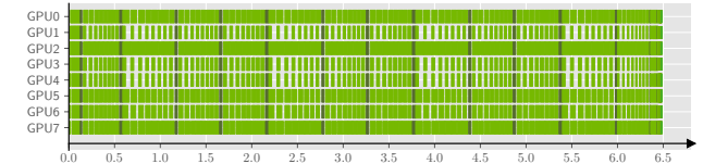
Figure 7: Timing profile for one frame of the museum model, using 8k \times 8k pixels and 8 paths/pixel, wave-front merging is enabled. Dark green indicates shading, light green indicates trace and cycle.
