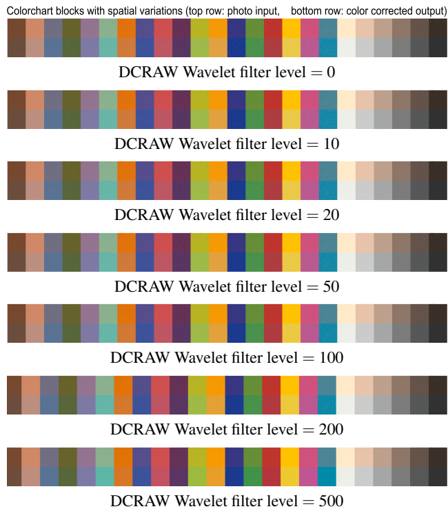
Figure 13: Examining proposed method for robustness against different levels of input chromatic noise in the input photo. CanonDarkroom_01.CR2 is subject to different levels of wavelet filtering by DCRAW to smooth out spatial noises. In each case, our method produces subjectively similar impressions about noise intensity as well colorful variations in each patch.
