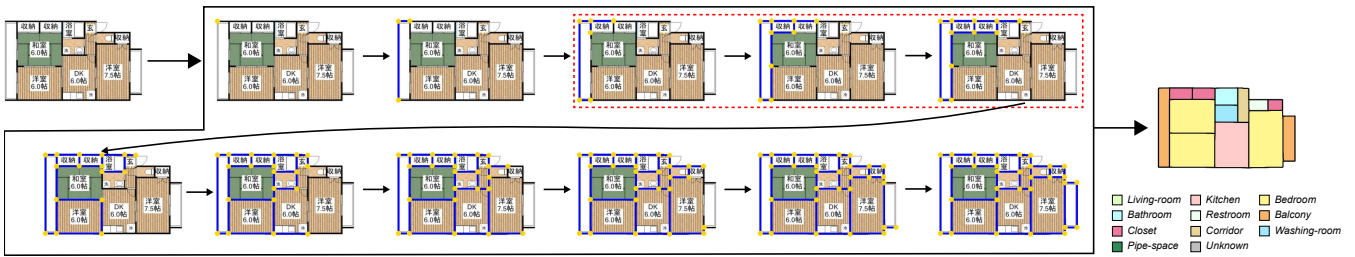
Figure 3: Overview of Raster-to-Graph. We represent the vector floorplan as a structural graph with semantics, and then the task of floorplan recognition can be viewed as structural graph prediction. Our method takes the rasterized floorplan as input, iteratively predicts nodes (shown in yellow) and edges (shown in blue) of the structural graph in the order of graph traversal, and finally obtains a complete structural graph. A vectorized floorplan can be easily extracted using the structural graph. It's worth noting that during the iterative process, our framework does not strictly adhere to the fixed order of graph traversal, as indicated in red. This is due to our training strategy, which allows a non-fixed order, a more general graph traversal, enhancing the flexibility of our prediction process.
