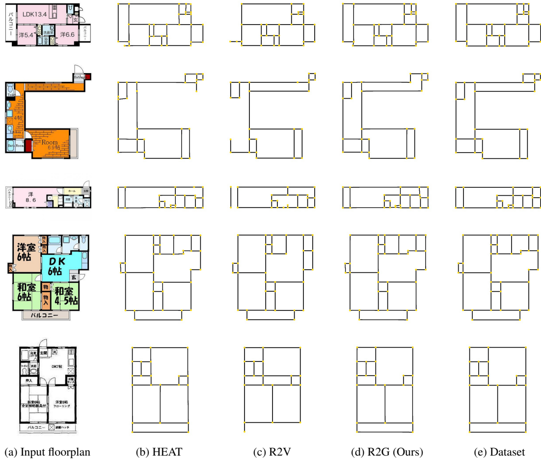
Figure 8: Qualitative evaluation on structural reconstruction. From (b)-(e), all columns are shown in vectorized floorplans. In (e), we present the corresponding "ground truth" in our dataset.
