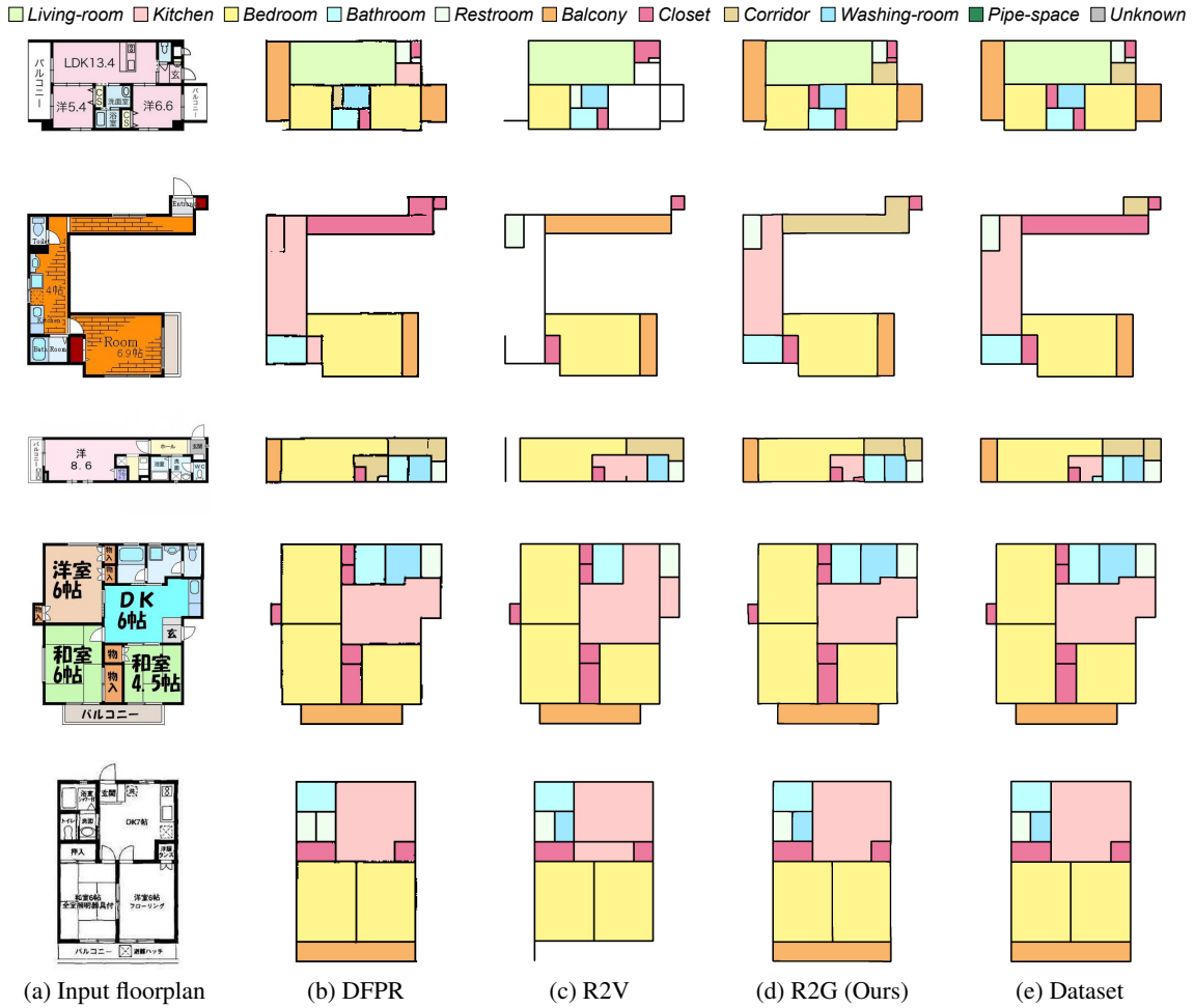
Figure 9: Qualitative evaluation on semantic recognition. From (b)-(e), only closed polygons are colored as rooms. In (e), we present the corresponding "ground truth" in our dataset. Note there might be a minor level of annotation errors in the semantic labeling of our dataset.
