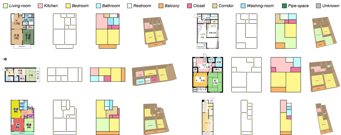
Figure 1: We propose a novel floorplan vectorization framework for recognizing the semantics and structures of rasterized floorplans. Here shows a gallery of rasterized floorplans and the corresponding vectorized results obtained through our framework. For each group, from left to right: a given rasterized floorplan, a structural graph obtained by our method, a vectorized floorplan with various colors representing different categories of rooms and a popup 3D model of the floorplan.
