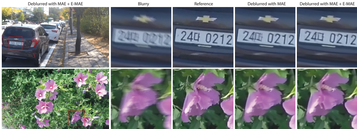
Figure 8: Visual results for the motion deblurring task when employing MAE and MAE + E-MAE as loss functions.
