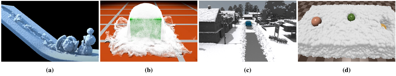
Figure 5: Snow simulation methods with their grid resolution/particles used to generate the image (a) packing snow effect captured by the MPM by Stomakhin et al. [SSC*13] ( 200 \times 240 \times 470 / 7.2M ), (b) hybrid particles and grid-based friction and cohesion by [TFN14] ( 50 \times 50 \times 50 / 33K ), (c) elastic deformation produced by the implicit compressible SPH solver of [GHB*20] ( -/2.57M ), (d) interactive/real-time snow simulation using iterative DEM solver on the GPU by Goswami et al. [GNN22] ( -/96K ).
