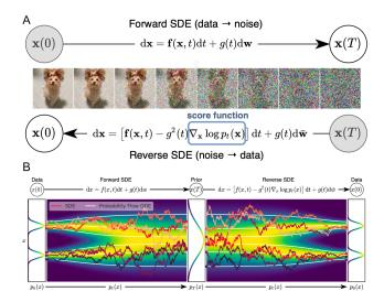
**Figure 2:** Diffusion Process. (A) The forward SDE transforms images to noise. The forward SDE can be reversed [And82] if we can predict the score function, enabling image synthesis. (B) The distributions of images and noise are linked with stochastic trajectories, modeled by SDEs, and deterministic trajectories, modeled by a probability flow ODE. Figures adapted from [SSDK\*20].
