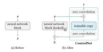
**Figure 4:** Overview of ControlNet. ControlNet [ZA23] modifies existing network architectures by duplicating network blocks and connecting them through zero convolutions. The auxiliary module takes some conditioning **c**, allowing the model to learn additional control handles.
