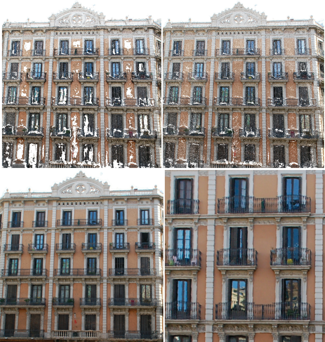
Figure 10: Impact of depth map repairing: point cloud from original depth maps, point cloud from repaired depth maps, reconstructed mesh, and close-up view with projective texture mapping.
