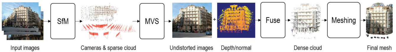
Figure 1: Standard pipeline for 3D reconstruction from images.
