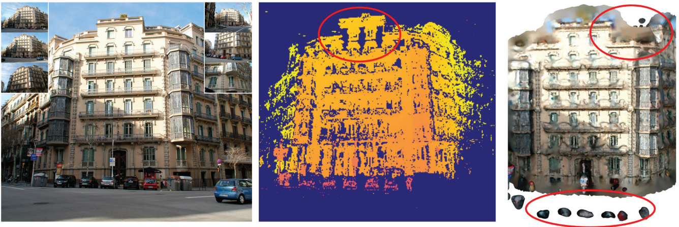
Figure 2: Artifacts in standard SfM+MVS pipelines: input images, depth map and final mesh.
