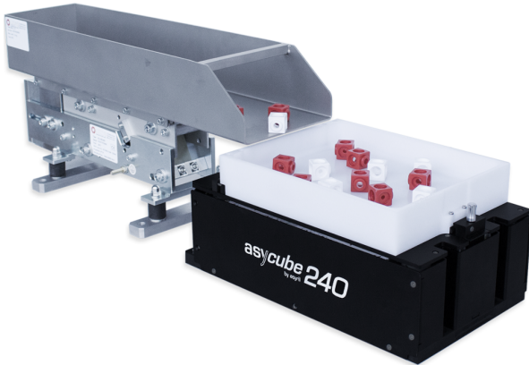
Figure 2: Commercial vibrating table ©Asyryl Asycube 240, Switzerland (source Asyryl).
