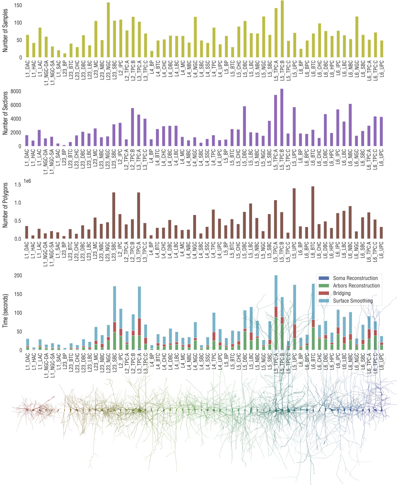
Figure 12: Performance profiles representing the time (in seconds) of reconstructing surface meshes with our method for a set of exemplar neuronal morphologies reflecting 60 various types of cortical neurons [MMR*15]. The profiles are shown with respect to the number of morphological samples, number of morphological sections and number of polygons in the reconstructed mesh to complete the analysis.
