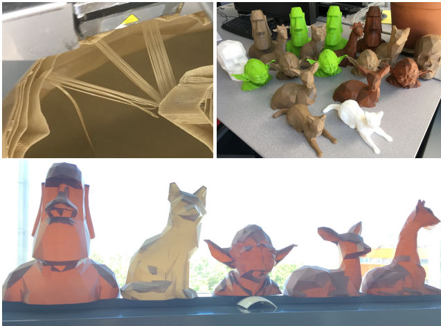
Figure 3: Top left. An unusually high number of bridges appears during the printing of the Fawn model. Top right. The models used for comparing with the work of Lee et al. [LL16]. Bottom. Printing without inner shell makes the models transparent enough to let us see the inner cavities.
