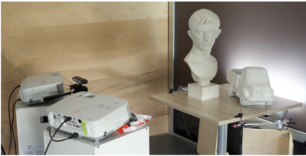
Figure 2: The setup for our multi-projector system. Two projectors and a depth camera are directed at the Augustus bust and a truck.
