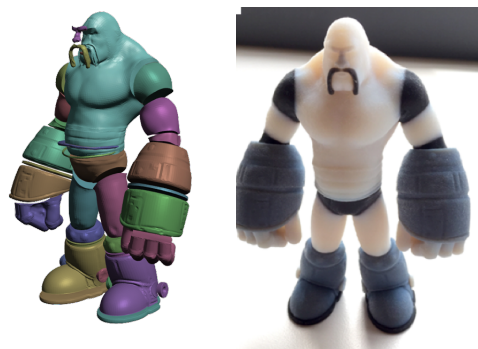
Figure 1: Left: exploded view of a non-manifold 3D model created with our system. Right: physical object fabricated with a multi-material 3D printer. White regions are hard solid plastic, and black regions are a flexible, rubber-like material.
