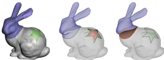
Figure 3: Two methods for creating non-manifold surface meshes from sets of selected faces. Center: offset the selected faces into the object. Right: fill the loop of boundary edges between two different triangle groups.
