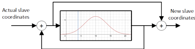
Figure 3: Gaussian backward feeding smoothing system.
