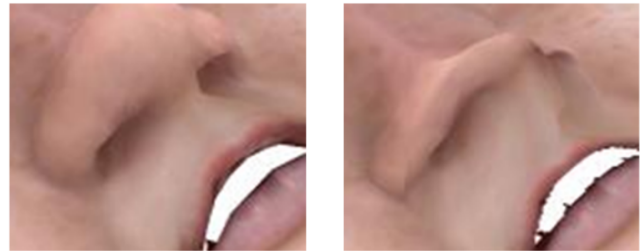
Figure 2: Example of viewpoint-dependent distortion of nose and mouth imagery resulting from a small rotation of a virtual object. The left pane shows a simulated view of the virtual object while the right pane shows the same view of one possible augmentation resulting from that pose of the virtual object being displayed on a static physical display surface corresponding to the un-rotated state of the virtual object.
