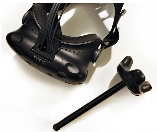
Figure 2: The HMD shown with the wand that is used to control the virtual ring and rod.
