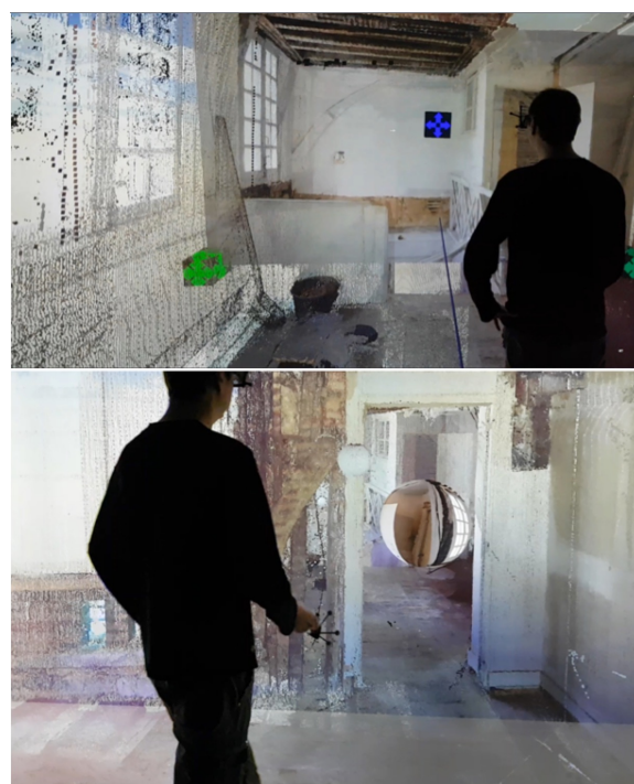
Figure 4: Top: Positioning of a photo within the VR application. Bottom: A floating sphere indicates a point of view of a photo in the application.
