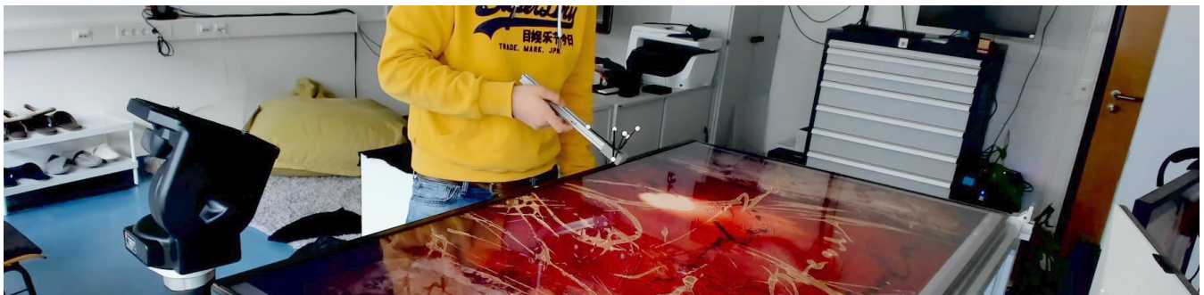
Figure 1: A user interacting with the proposed tabletop system to inspect the design and glossiness of a decorative surface. He holds a physical proxy of a virtual light source that can be used to illuminate the virtual scene on the display.
