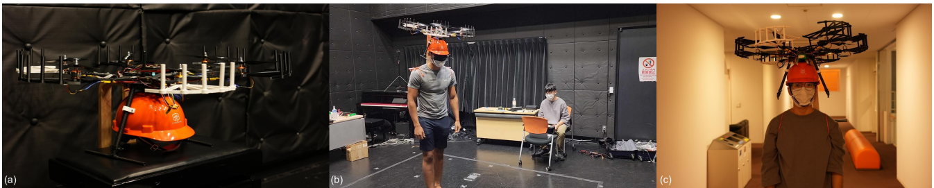
Figure 1: a) Prototype image of HumanCopter b) Image of navigation experiment c) a front view for HumanCopter
