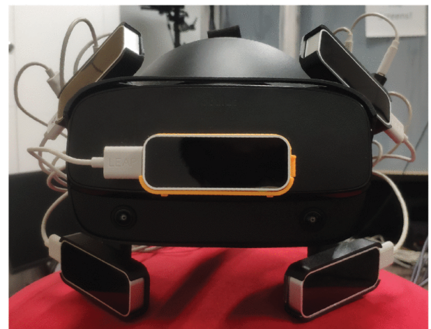
Figure 2: The setup for the Multi Leap Motion system strapped on an HMD. [WWJ*21]
