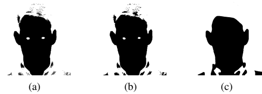
Figure 5: Post-processing skin detection. a) initial skin detection, b) after morphological cleaning, c) after mapping colours to the dominant skin colour.
