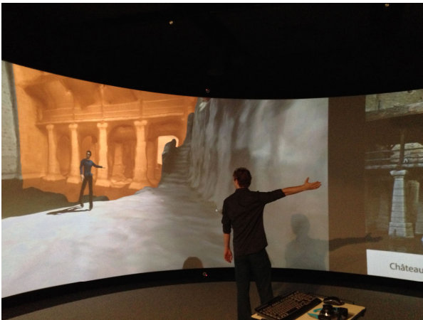
Figure 2: The avatar mirrors the speaker's tracked gestures, triggering slides by pointing at the relevant object.
