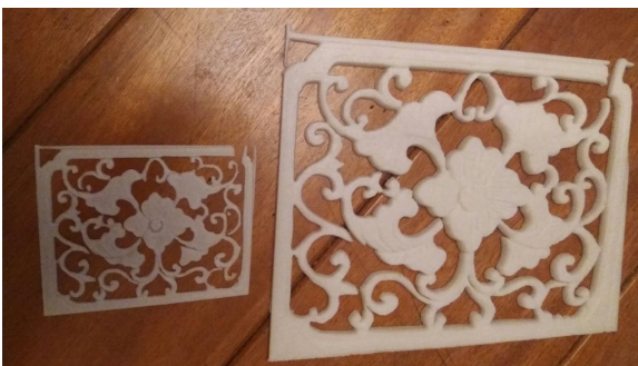
Figure 11: 3D printing of 3D mesh produced by using a depthmap of the digital photographs.
