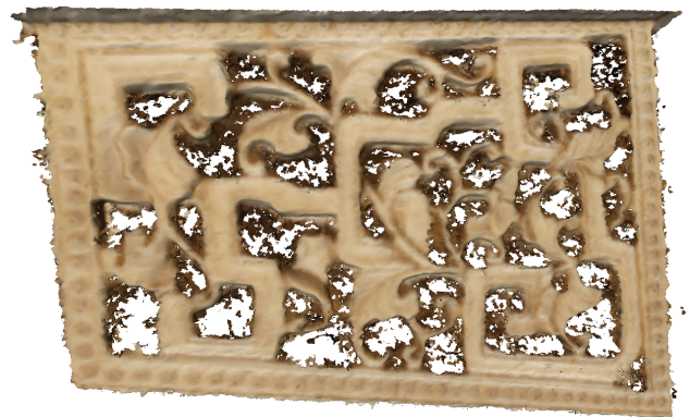
Figure 6: A resulting 3D model of a window panel using photogrammetry techniques. At a first glance the acquired point cloud would attend the demands, but underlying noise always entailed in low quality geometric reconstructions.
