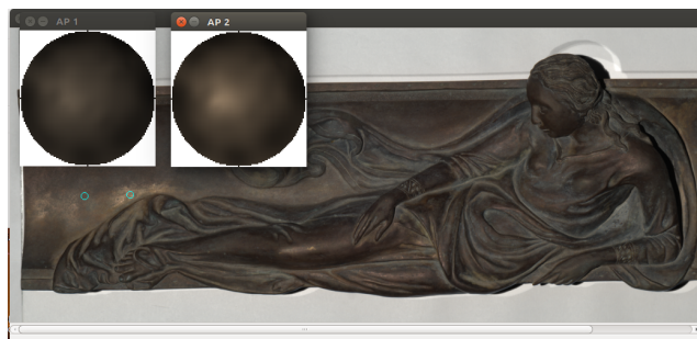
Figure 8: The RTI analysis interface allows the display of a reflectance image related to single point or ROI, allowing an easy comparison of different material properties.
