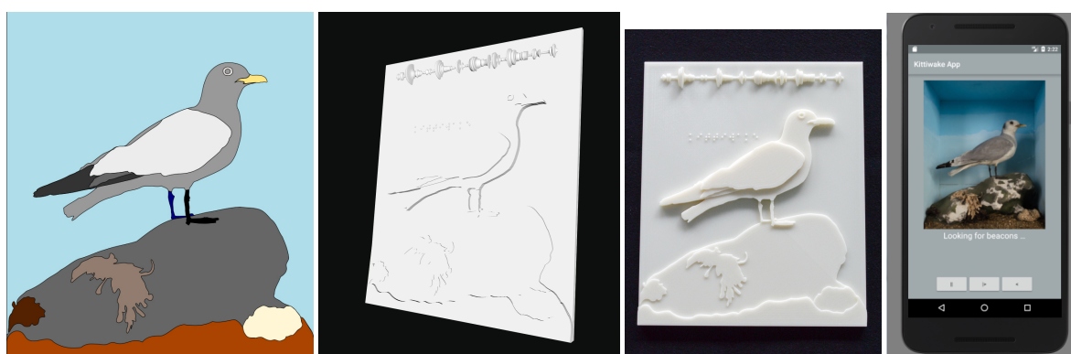
Figure 1: a) Vector graphic representation of the kittiwake “diorama”; b) 3D relief model generated from scene; c) 3D print of relief; and d) context-aware mobile application for enriching museum experience of visually impaired visitors.
