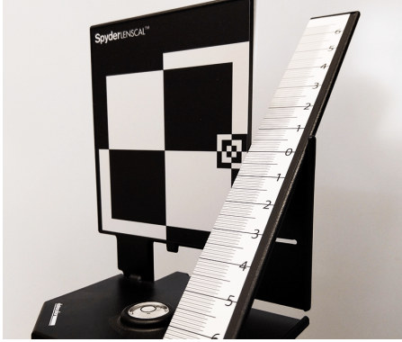
Figure 1: Calibration object. For our experiments we used a commercially available product designed for autofocus calibration.
