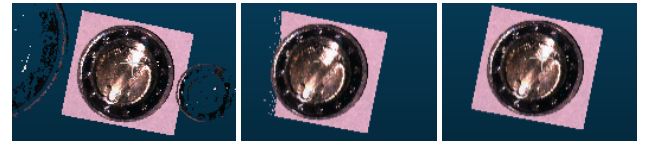
Figure 8: Outliers in the unfiltered point cloud (left), after applying the Interquartile range filter (middle) and after alignment of the point cloud using a principal component analysis, followed by application of Interquartile range filter (right).
