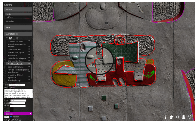
Figure 11: Annotation authoring. The tool, based on the viewer, allows users to draw over the model, place pins, and control all rendering, viewing, and lens positioning settings associated to the annotation. Moreover, annotation description and hierarchical annotation ordering are also defined.
