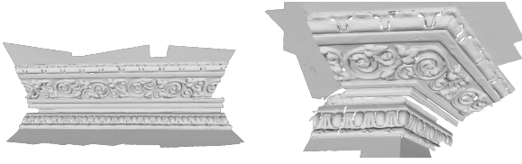
Figure 10: Resulting 3D models both of linear and corner pattern containing the different mouldings that need to be fabricated
