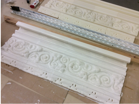
Figure 13: Assembled section of the cornice fabricated using additive manufacturing technologies
