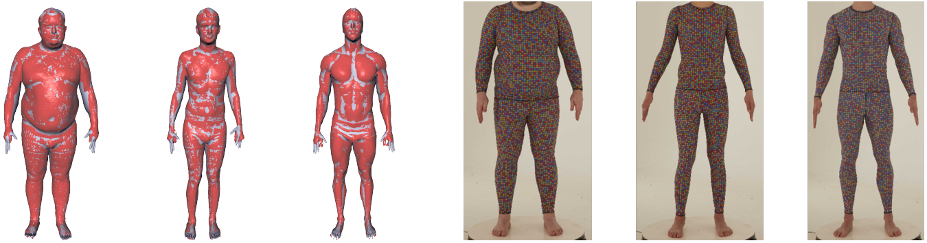
Figure 9: Left: Registration Results for three test persons. The template (gray) is deformed to best match with the scan (red). Right: The made-to-scan developed prototype suits made of a fabric with color pattern.
