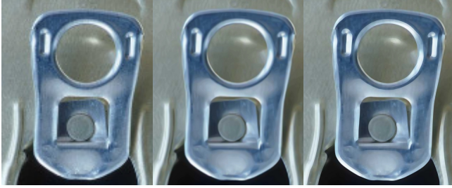
Figure 14: Both IRT (right) and 9X superresolution (middle) reduce blurring and aliasing near edges; such artifacts are symptomatic of the bilinear interpolation (left).
