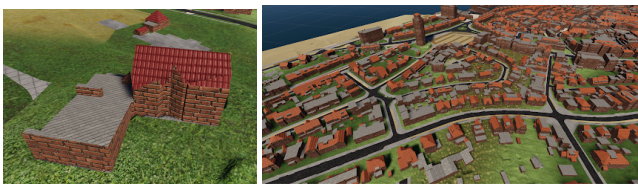
Figure 3: Left: Texture mapping for building facades. Right: Building model implementation for Zandvoort, The Netherlands.
