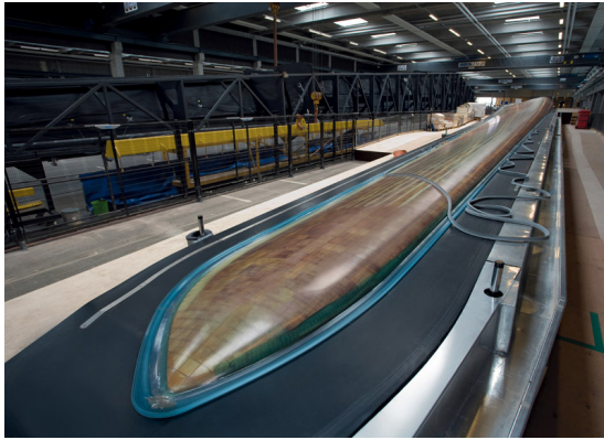
Figure 3: Wind turbine blade right after molding.
