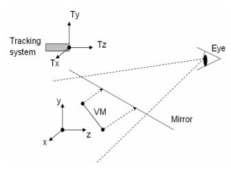
Figure 2: System's and Tracking coordinate systems
