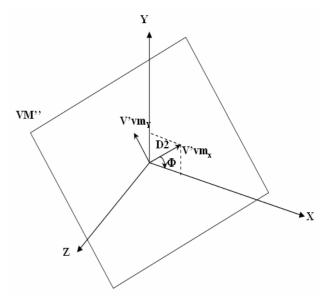
Figure 5: Second Rotation for the virtual monitor to be normal to the Z axis
