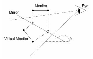
Figure 1: Mirror refection of the Monitor
