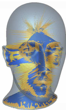
Figure 8: The inner Voronoi diagram subset V of the head figure and the set of faces that are removed (yellow) in order to arrive at an approximated medial axis M (blue).
