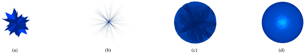
Figure 10: (a) The approximated medial axis of a ball enlarged by a factor of around 100 (b) The face-vertex pyramids of the ball: note there are much fewer such pyramids than in the case of the non-filtered Voronoi. (c) The paths of edge-edge tetrahedra added between the key vertices of the boundary (d) The solid ball with all tetrahedra.
