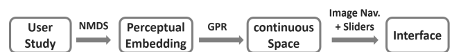
Figure 1: The pipeline of our method. We collect triplet comparison data from a user study and convert them into perceptual embedding using NMDS. Next we use GPR interpolation to connect the embedding and the tabulated BRDF to build a continuous perceptual space, based on which we propose a new interface for editing.
