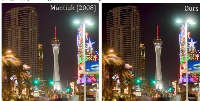
Figure 9: Tone mapped images using Mantiuk’s [MDK08] original tone mapping operator (left), and plugging our CSF model (right). For scenes with dark surround luminances, our CSF presents a low sensitivity, therefore it compresses contrast better leading to cleaner images with less residual haze (better seen in the digital version).
