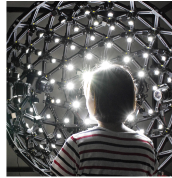
Figure 5: LED hemisphere for illuminating a subject with polarized spherical illumination.
