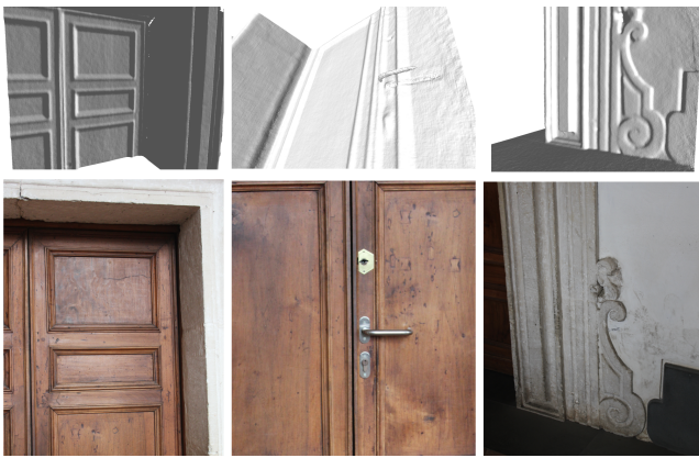
Figure 1: View of the Structure Sensor behavior on three different materials (from left to right): wood, metal, limestone.
