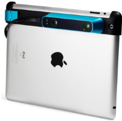
Figure 8: Structure sensor clipped onto an iPad.
